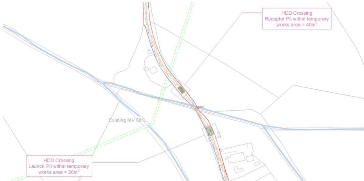
Figure 19 - Bridge 2 HDD Crossing on with Tailte Eireann Background
